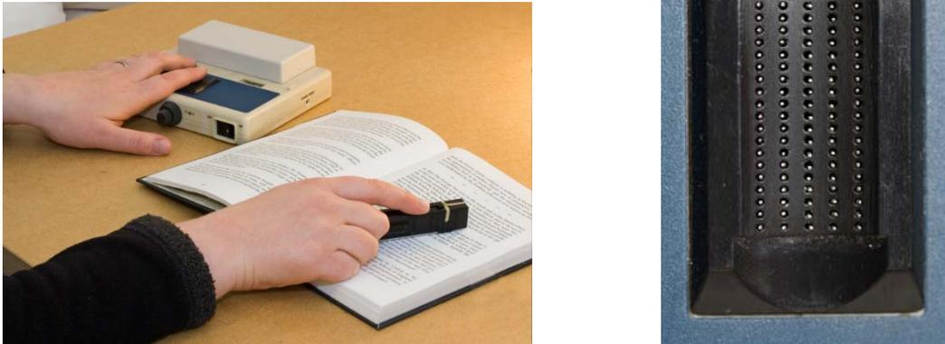
Figure 3. Using the Optacon device to read text. The image on the right shows a close-up of the pin array.
