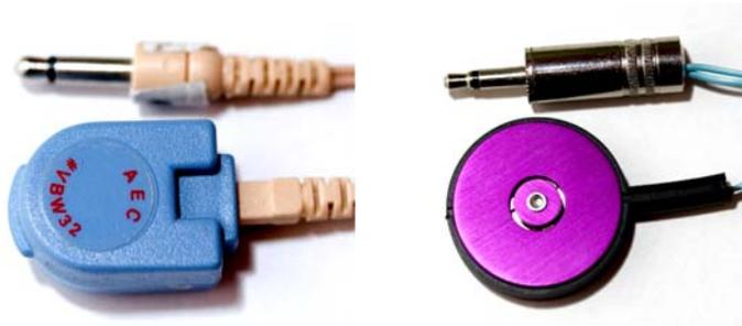
Figure 2: Left – a TACTAID VBW32 transducer, right an EAI C2 Tactor.
