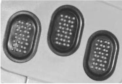
Figure 1. A tactile pin array for fingertip display, consisting of three 4 x 8 arrays of pins.
