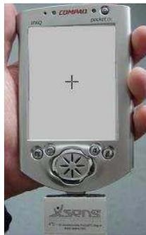
**Figure 2: A Compaq iPAQ handheld computer with an Xsens 3-axis accelerometer for detecting device movements ([www.xsens.com](http://www.xsens.com)).**
