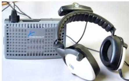
**Figure 1: A simple wearable computer system comprising a Xybernaut MAV wearable computer, a pair of standard headphones and an Intersense orientation tracker for detecting head movements (on top of the headphones) [7].**
