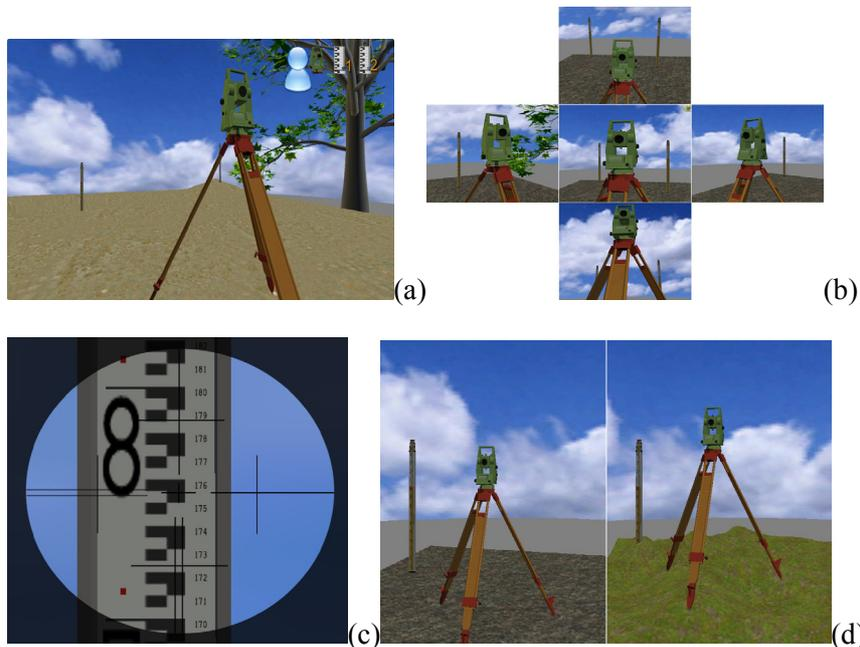
Figure 5. Screenshots of SimuSurvey X: (a) in the navigation mode, icons in the upper-right corner show the controlled object, (b) views of the object at different angles (c) observation through the telescope on the instrument, (d) the height of the object alters according to the terrain.
