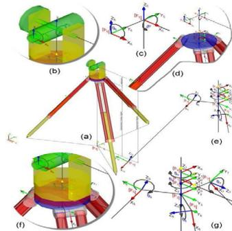
Figure 3. The analysis of the kinematics model of the surveying instruments
