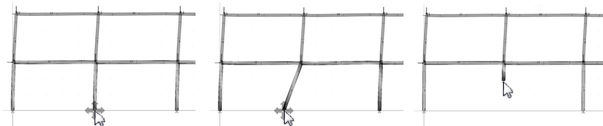
Figure 2. Dragging a node in the frame system (re-analysis time: 70 ms on a standard PC)
