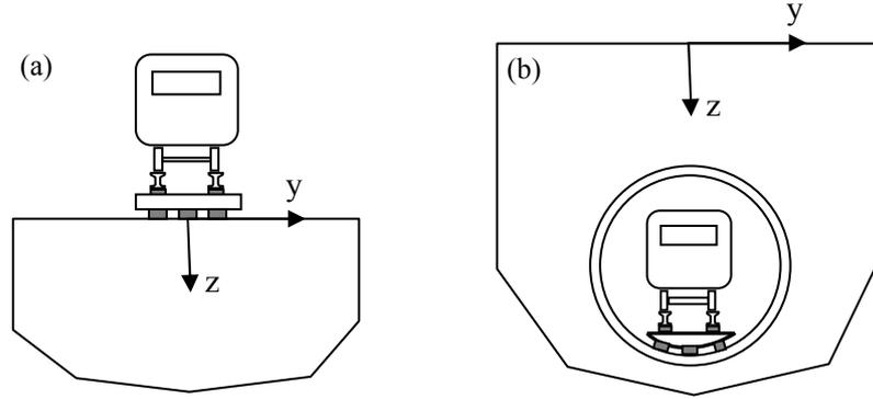
Figure 1. Vibration due to moving trains on floating-slab tracks is calculated at the free surface, i.e. at  $z=0$ , for (a) surface and (b) underground railway tracks. Resilient elements (i.e. railpads and slab bearings) are shown in dark colour
