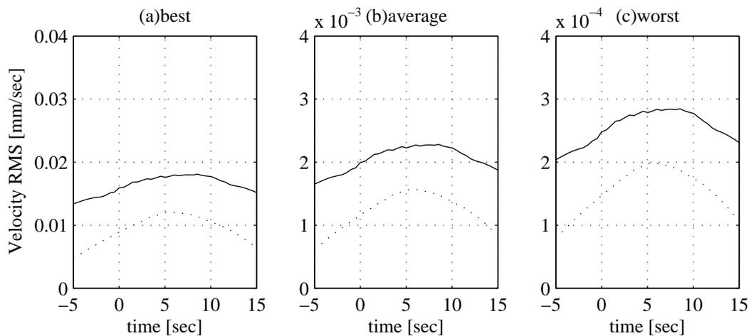
Figure 3. The vertical velocity RMS at a point at the free-surface at 40m distance from the track due to train moving on a (-) surface track and (...) underground track with a given rail roughness spectrum as described by (Frederich, 1984) for best, average and worst conditions
