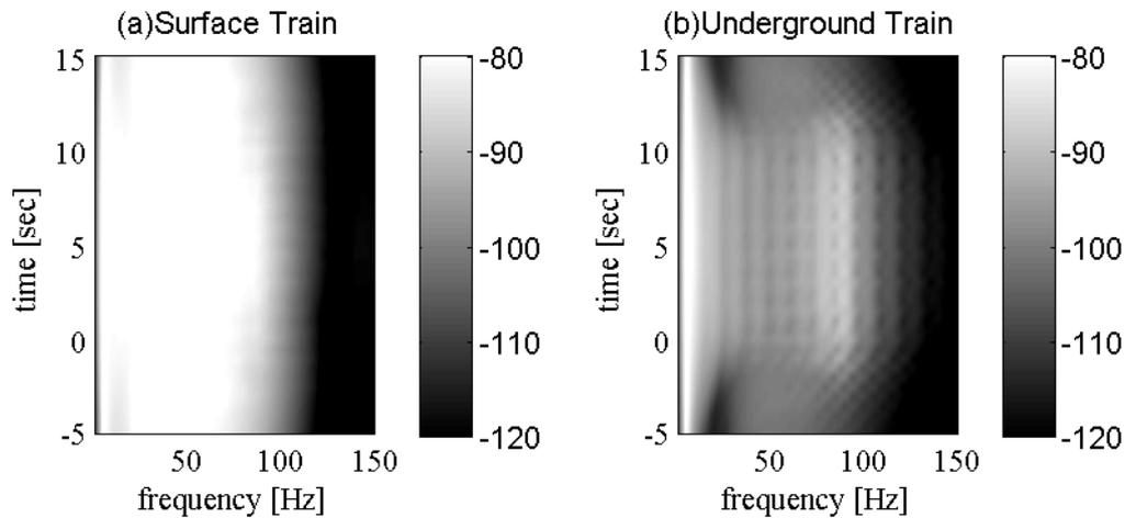
Figure 2. The PSD of the vertical displacement at a point at 40m away from tracks due to a train moving along a track with white-noise rail roughness
