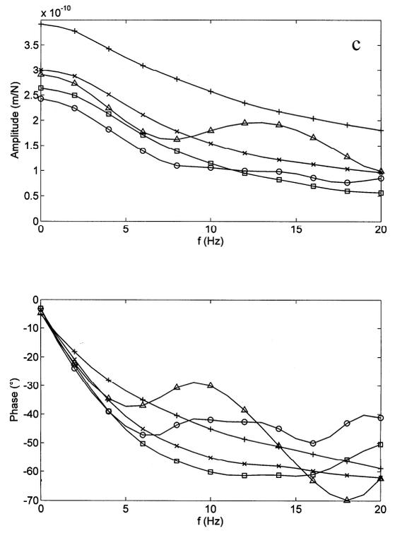
Figure 1. Amplitude and phase of the a) vertical rigid, b) vertical flexible, c) horizontal compliance of different pile groups  $\square$  grid,  $\circ$  circle,  $\triangle$  parallel lines,  $\times$  cross and  $+$  line, concrete piles of  $L = 20$  m,  $R = 0.5$  m, continuum soil with shear wave velocity  $v_s = 200$  m/s.
