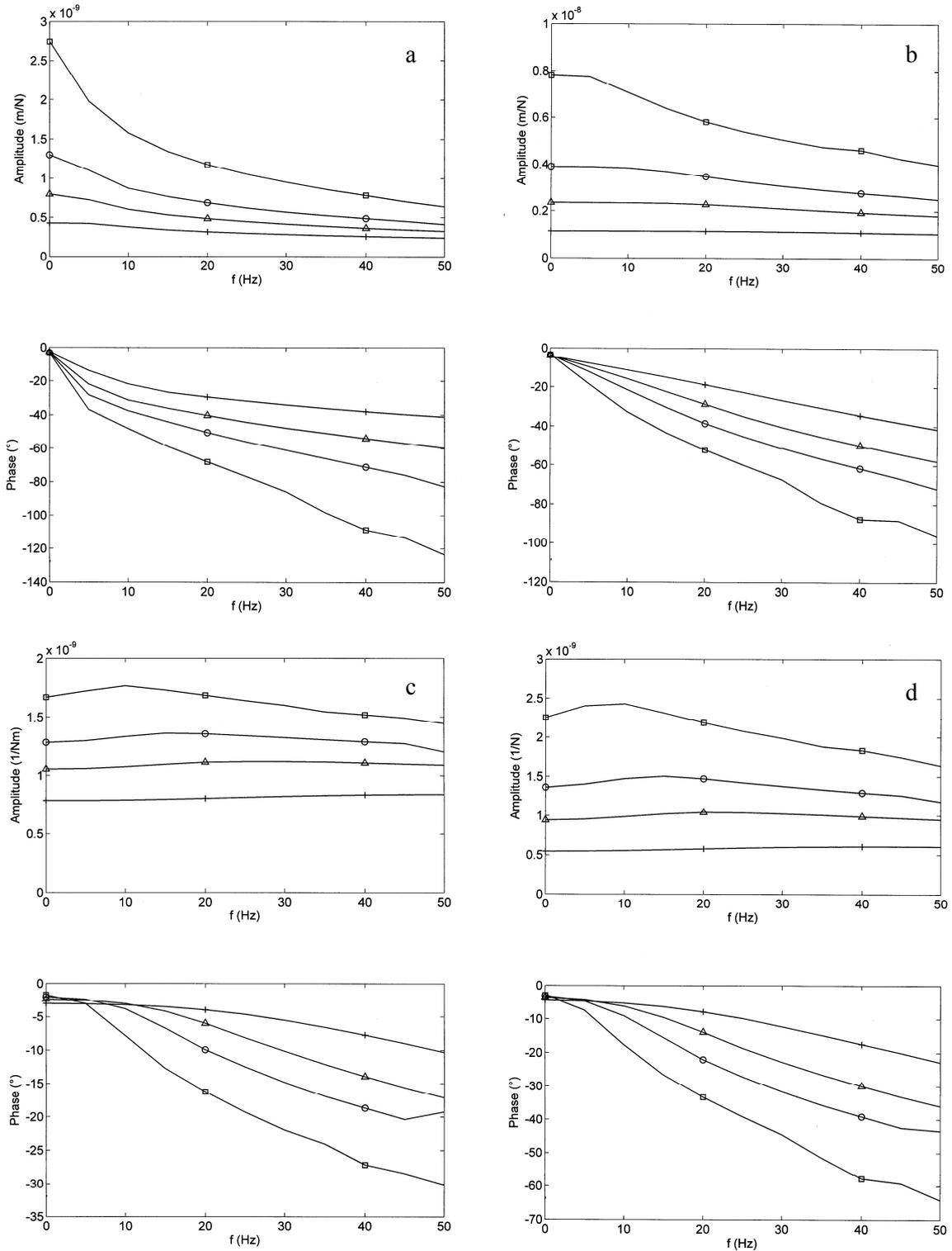
Figure 2. Amplitude and phase of the a) vertical, b) horizontal, c) rocking, and d) coupling compliance of concrete piles ( $L = 10$  m,  $R = 0.5$  m) on different continuum soils with  $v_s = \square 100, \circ 150, \triangle 200, \times 300$  m/s.
