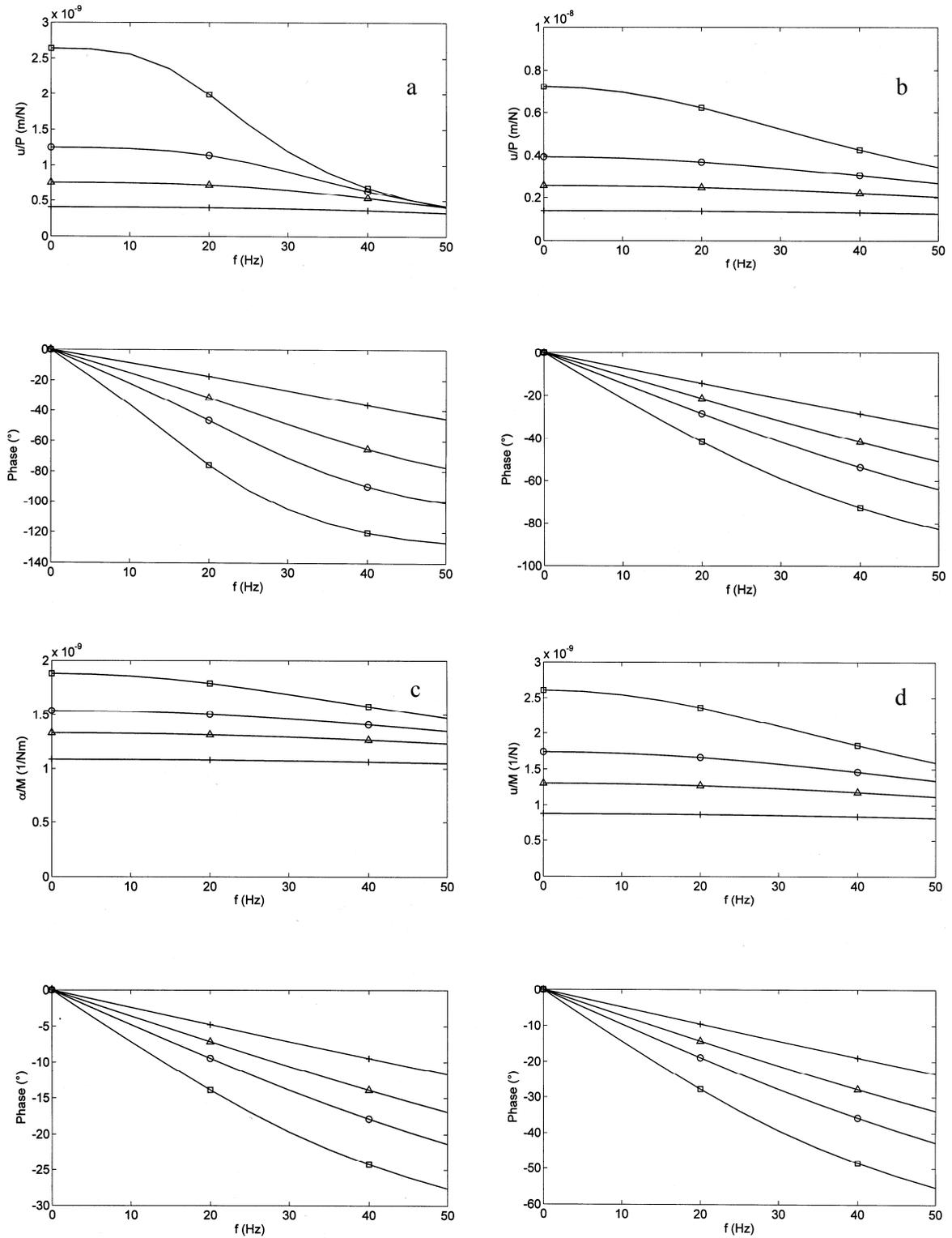
Figure 3. Amplitude and phase of the a) vertical, b) horizontal, c) rocking, and d) coupling compliance of infinite concrete piles ( $R = 0.5$  m) on different Winkler soils with  $k' = \square, \circ, \triangle, \times 9 \cdot 10^8 \text{ N/m}^2$  and  $c' = \square, \circ, \triangle, \times 2.4 \cdot 10^6 \text{ Ns/m}$ , a) vertical finite pile of  $L = 10$  m, and with lower Winkler parameters  $k' = 2G$ ,  $c' = 4\rho v_s R$ .
