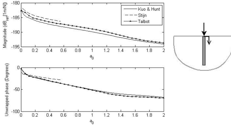
Figure 1. The vertical driving point response of a pile subjected to unit harmonic excitation in the z-direction.
