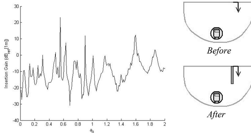
Figure 4. Vertical insertion gain for a 20m pile located 10m from an underground railway.
