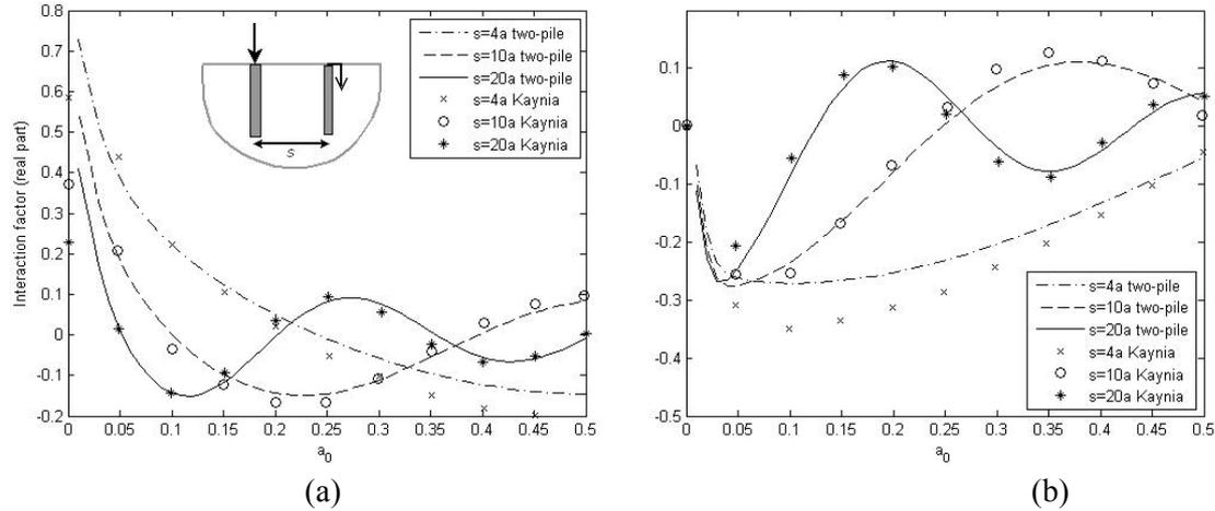
Figure 3. (a) Real part; and (b) imaginary part of the axial response of a finite pile using the two pile model.
