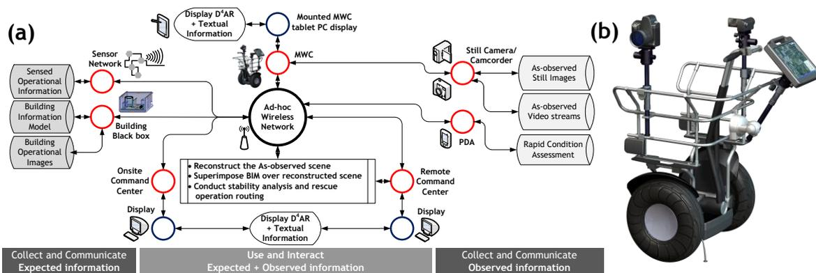
Figure 1, (a) An overview of the proposed approach, data flow and data collection, analysis and communication technological components. (b) MWC provides the ability to carry and use data collection and communication equipment during rapid response to XEs.
