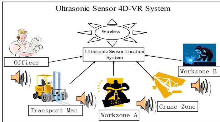
Figure 2. Sketch map of safety control system of ultrasonic sensor + 4D VR safety-training system
