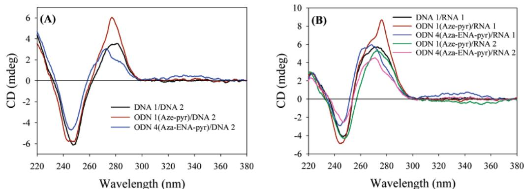
**FIGURE 6.** (A) CD spectra of duplexes formed by native DNA 1 with complementary DNA 2 and Aze-pyr (X)-modified ODN 1 and Aza-ENA-pyr (Y)-modified ODN 4 with complementary DNA 2. (B) CD spectra of duplexes formed by native DNA 1 with complementary RNA 1 and pyrene-modified ODNs 1 and 4 with complementary RNA 1 and with RNA 2 containing single base (G) mismatch. The total strand concentration was 10  $\mu\text{M}$ .
