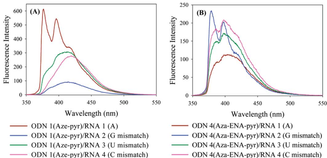
**FIGURE 4.** Fluorescence emission spectra of (A) Aze-pyr (**X**)-modified ODN **1** and (B) Aza-ENA-pyr (**Y**)-modified ODN **4** hybridized to the complementary RNA **1** and single base mismatch (**G**, **U**, or **C**) RNA **2**, RNA **3**, and RNA **4**, respectively. Spectra were recorded at a total strand concentration of  $0.8 \mu\text{M}$  and with an excitation wavelength of  $340 \text{ nm}$ .
