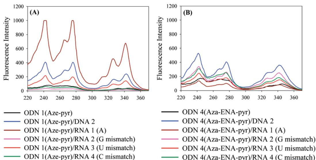
**FIGURE 5.** Fluorescence excitation spectra of (A) Aze-pyr (X)-modified ODN 1 and (B) Aza-ENA-pyr (Y)-modified ODN 4 and the corresponding duplexes with complementary DNA 2, complementary RNA 1, and single base mismatched (G, U or C) RNA 2, RNA 3, and RNA 4, respectively, obtained by monitoring wavelengths at (A) 376 nm and (B) 380 nm. Spectra were recorded at a total strand concentration of 0.8  $\mu\text{M}$ .
