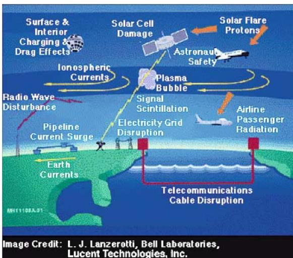
**Figure 5.** Some of the effects of solar activity on technical systems deployed on the Earth's surface and in space.
