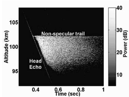
**Figure 1.** Altitude-time-intensity image of a head and subsequent non-specular echoes over extended range from ALTAIR VHF Radar. The diagonal line to the left is called a head echo, while the echoes spread in range and time to the right are the non-specular trail. Figure reproduced from Close et al. [2002].
