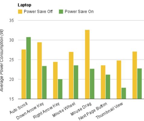
**Figure 3:** Average Power Consumption values for the Laptop Condition.
