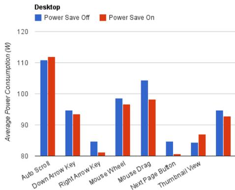
**Figure 2:** Average Power Consumption values for the Desktop Condition.
