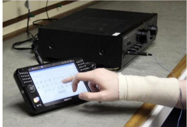
**Figure 6: Experimental setup. In this condition (Cw) the C2 is placed on the wrist using a tubigrip bandage.**
