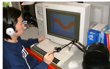
Figure 4 Audio-haptic line graph
