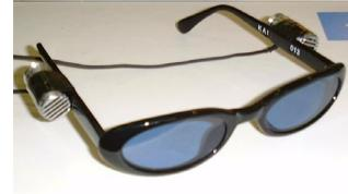
Figure 7 Pre-amplified microphones for capturing real world sounds
