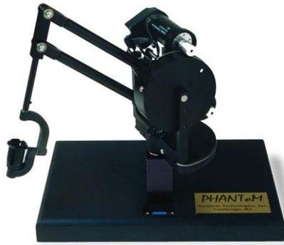
**Figure 1. PHANToM from SensAble Technologies Inc.**
