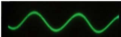
Figure 5: Output of TACTAID when a sine wave was played through it.
