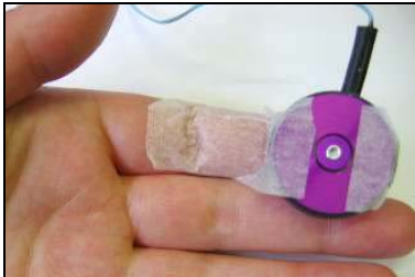
Figure 8: C2 Tactor attached to finger.
