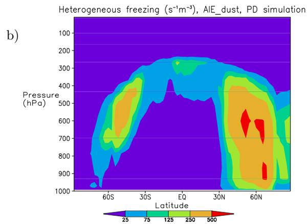
Figure 7: Rate of ice crystal production through heterogeneous freezing processes in a) AIE\_ctl and b) AIE\_dust, both from PD simulations.
