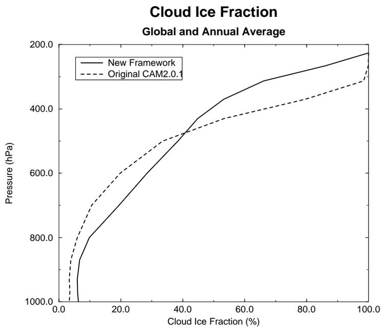
Figure 2: Global mean cloud ice fraction averaged over 5 years as calculated by the new framework for aerosol effects on ice clouds (solid line) and that of the original CAM2.0.1 method (dashed line).
