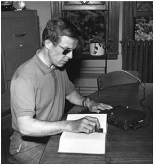
Fig. 3. Visually impaired person using the Optacon device to read text. The handheld camera detects light and dark areas of the page and converts to a vibrotactile representation, presented to the non-dominant hand on the pin array (Image used with permission from [www.carroll.org](http://www.carroll.org)).
