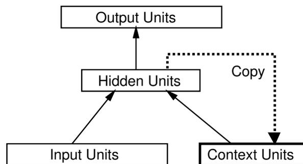
Figure 2: The recurrent network architecture of Elman.
