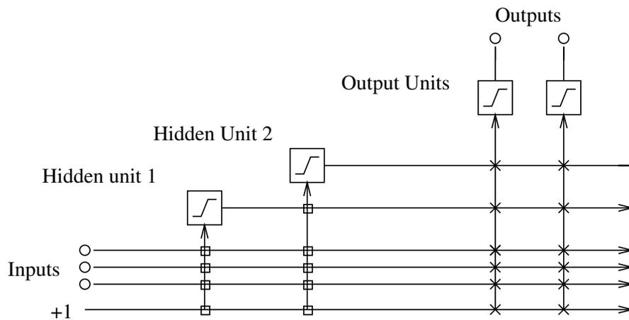
Figure 1: The Cascade-Correlation architecture after two hidden units have been added. The vertical lines sum all incoming activation. Boxed connections are frozen, X connections are trained repeatedly.
