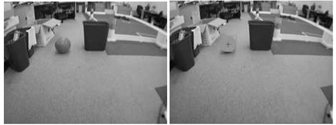
Figure 4. The left image shows the raw output from the camera in a lab setting. The right image shows the results after processing. 'Ball' pixels are shown as orange (shown in gray here), a bounding box is drawn around the resulting region, and its centroid is marked with a '+'.
