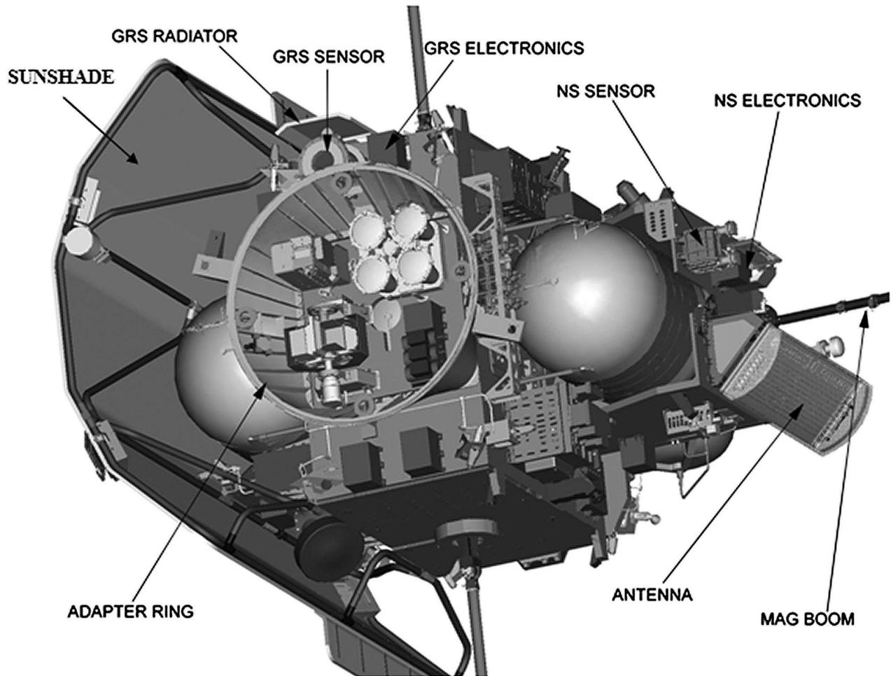
**Figure A3.** CAD drawing of GRS and NS as positioned on the MESSENGER spacecraft. Only a portion of the 3.6-m boom for MESSENGER's Magnetometer (MAG) is shown. Also indicated are one of MESSENGER's two high-gain phased-array antennas, the carbon fiber sunshade, and the adapter ring by which the spacecraft was mated to the upper stage of the launch vehicle. Figure reproduced from Rhodes *et al.* [2011].
