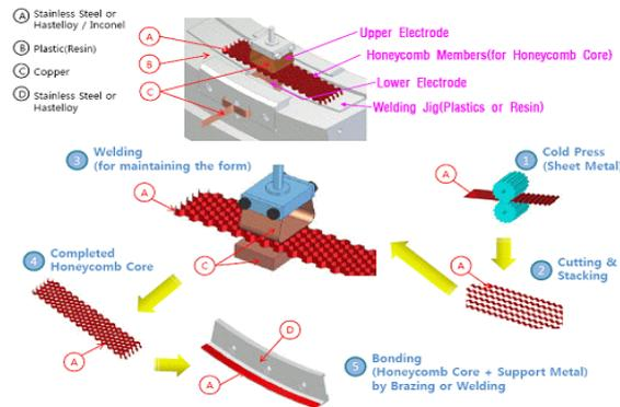
**Fig. 2.** Forming process to make honeycomb seal
