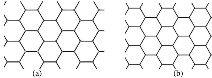
**Fig. 1.** Regular hexagonal honeycomb structure: (a) commercial honeycomb with curved walls at the intersection points; (b) theoretical honeycomb with straight walls
