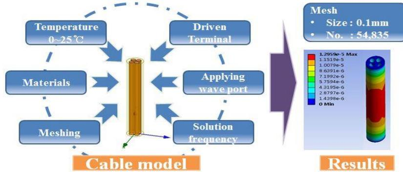
Fig. 1. Process of FEM analysis
