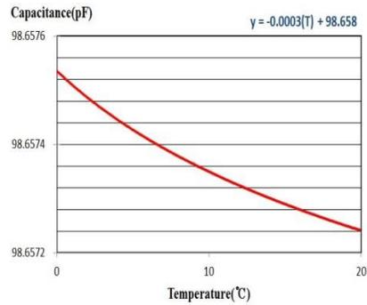
Fig. 5. Capacitance variation in cable
