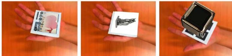
**Fig.1.** Contents Augmentation using Marker Array
