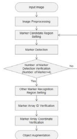
Fig.1. Contents Augmentation using Marker Array
