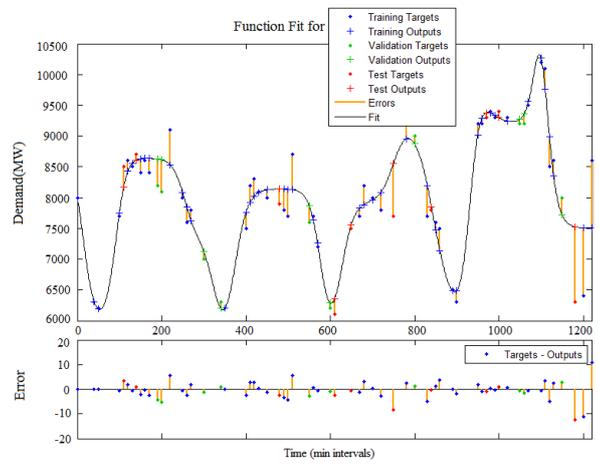
**Fig. 1.** Comparison of electricity load on the grid for four days in winter
