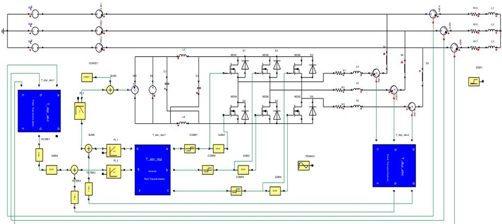
**Figure 4. Simulation model of the SVG system**
