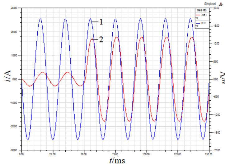
**Figure 6. Voltage and current compensation waveforms under 12V DC source supply**
