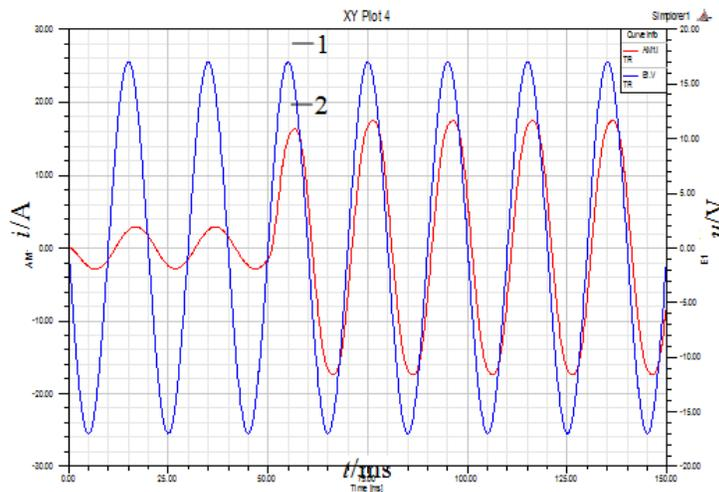
**Figure 5. Voltage and current compensation waveforms under 200 $\mu\text{F}$  capacitor supply**
