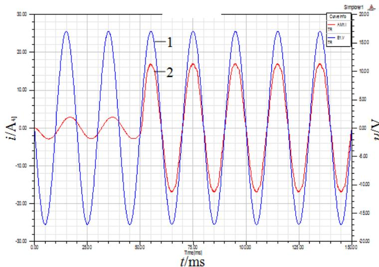
**Figure 7. Voltage and current compensation waveforms under Z-source network supply**
