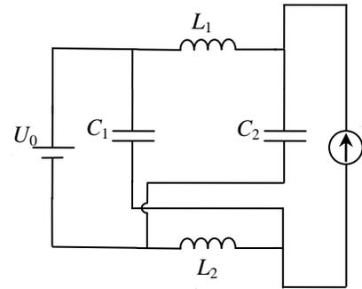
**Figure 2. Equivalent circuit at traditional state**
