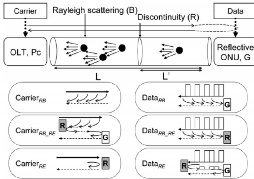
**Figure. 1 The module of link transmission system and the interference signals of the upstream direction**
