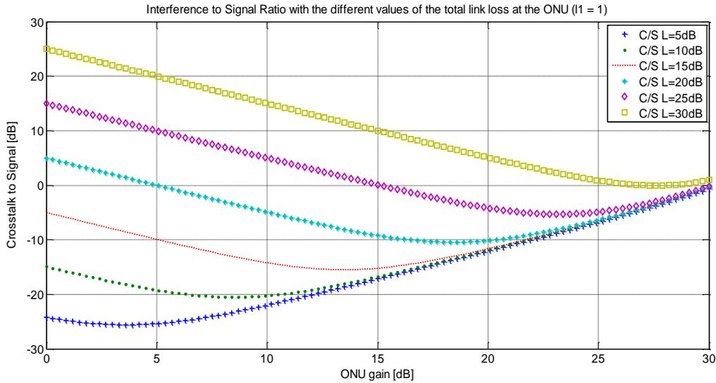
**Figure 8. Total crosstalk to signal ratio with some link loss and different gain**
