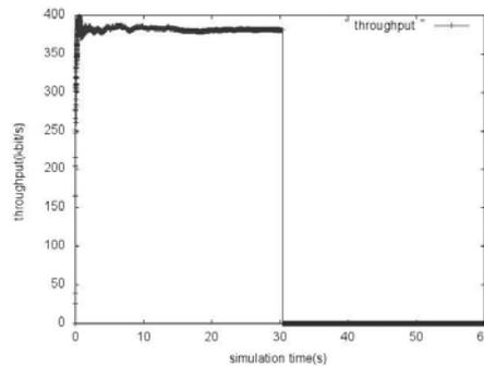
**Fig. 3.** Throughput of a sink related to a cluster's data (no data replication used)
