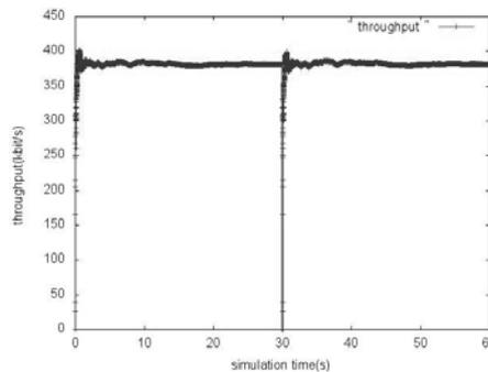
**Fig. 4.** Throughput of a sink related to a cluster's data (data replication used)
