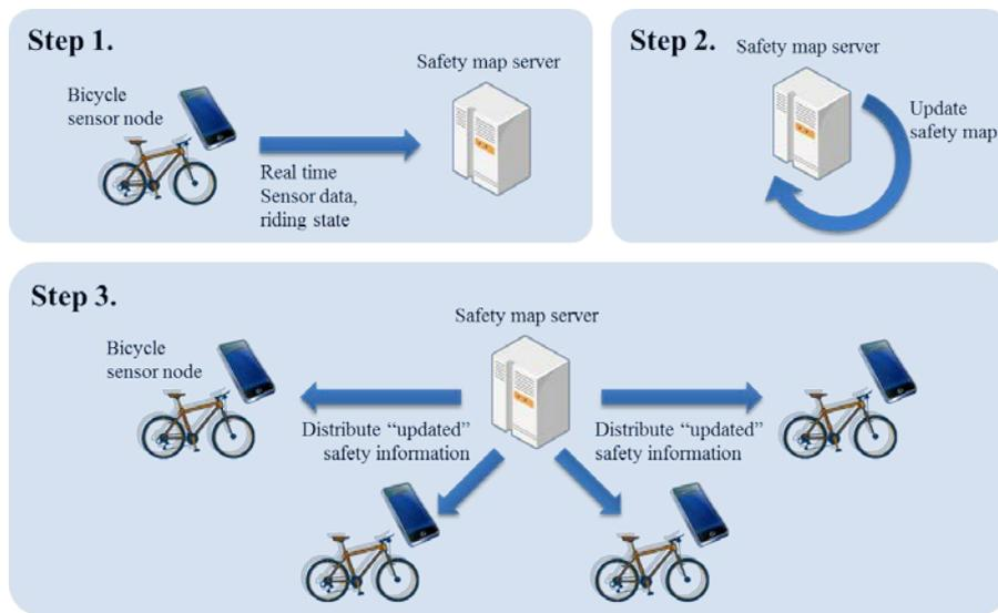
Fig. 1. Procedures and structure of self-updating bicycle safety map system
