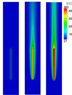
**Fig. 4.** Temperature characteristics of element according to time step; (a)  $t=0$  sec, (b)  $t=20$  sec, (c)  $t=100$  sec.
