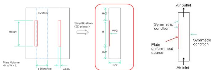
Fig. 3. Thermal analysis model and boundary conditions.
