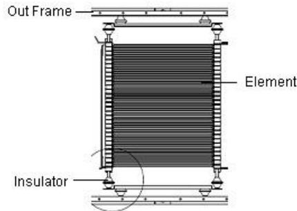
Fig. 2. Configuration of dynamic braking resistor.
