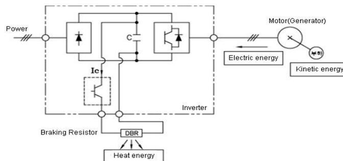
Fig. 1. Operating principle of regenerative braking by inverter.
