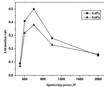
**Fig.3-3.** Attenuation rate of Ni film with different sputtering power
