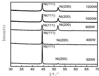
**Fig.3-1.** XRD patterns of films with different sputtering power
