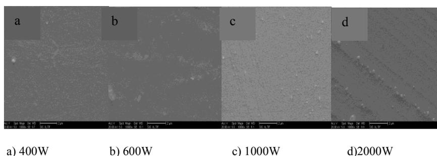
**Fig.3-2.** SEM images of Ni film with different sputtering power
