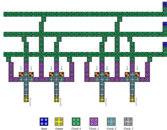
**Fig. 6:** Proposed structure of the QCA decoder.
