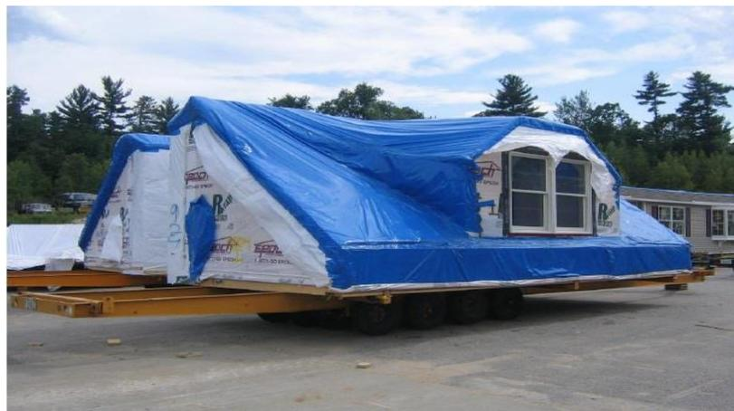
**Figure 21. Modules are Carefully Secured to the Truck**
