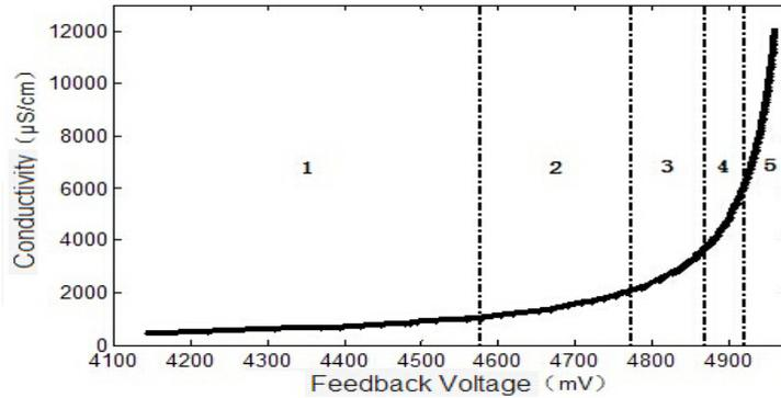
**Fig.3.** The conductivity and feedback voltage relationship diagram.
