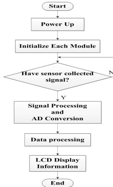
Fig.2. A Flow Diagram Design of the System.
