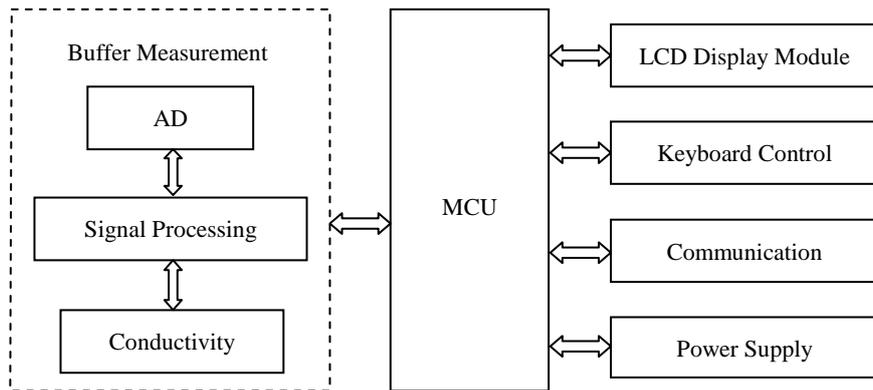
**Fig.1.** Hardware structure diagram of the measurement and transmission unit.
