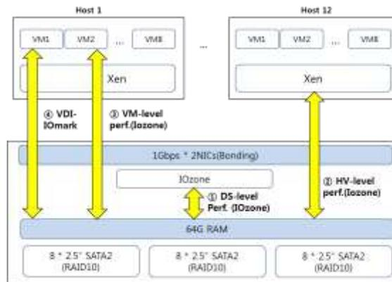
**Fig. 1.** System configuration and testing issues
