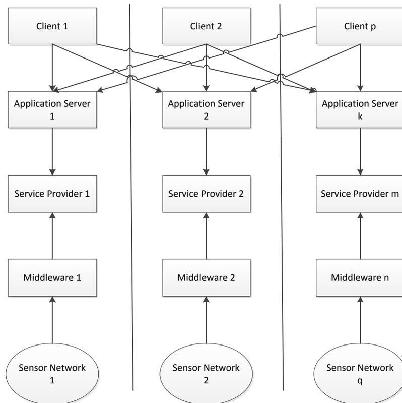
**Fig. 2.** Previous sensor web architecture based on middleware
