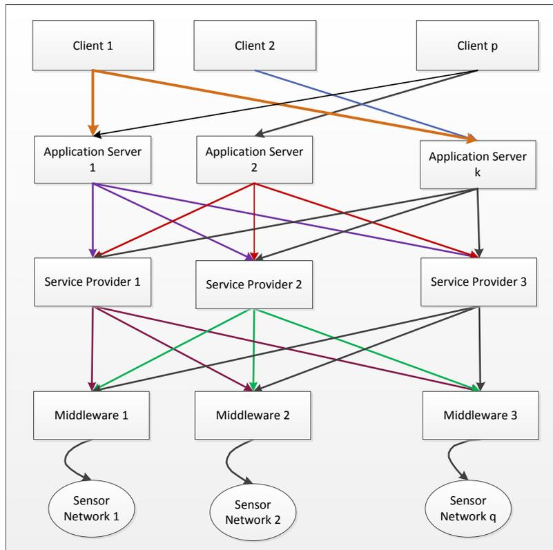
Fig. 1. Proposed Sensor Web architecture based on distributed middleware
