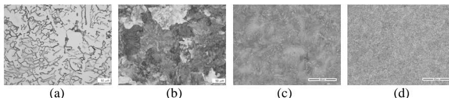
**Fig. 2.** Some examples of steel grade: (a) austenite (b) pearlite (c) martensite (d) ferrite
