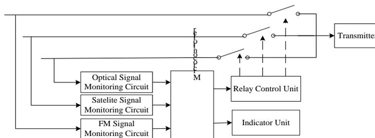
**Fig. 1.** The structure diagram of audio source switcher
