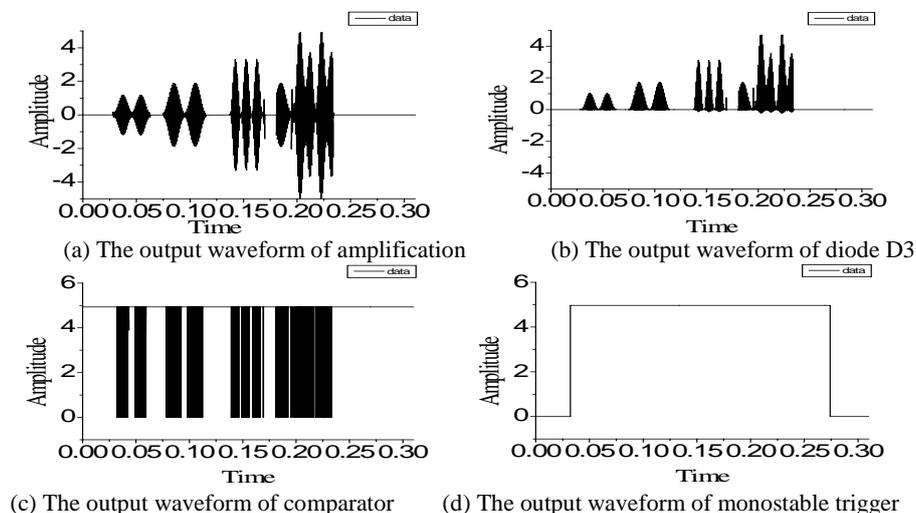
Fig. 4. The output waveform of circuit
