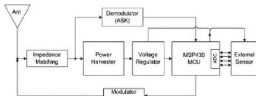
Fig. 2. RFID sensor tag block diagram
