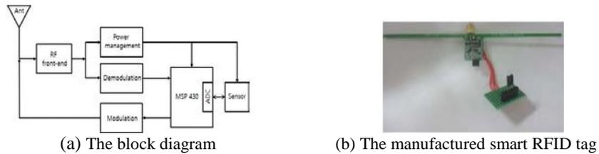
Fig. 1 Smart RFID tag system
