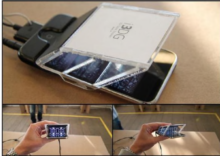
Fig. 1. The i3Dg accessory for iPhone utilizes three panes of plastic to create a multi-depth experience.
