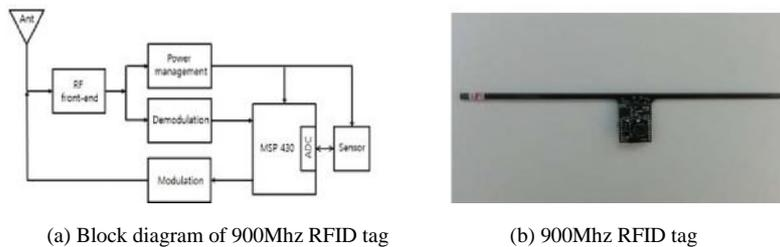
**Fig .2** Block diagram of 900MHz RFID tag
