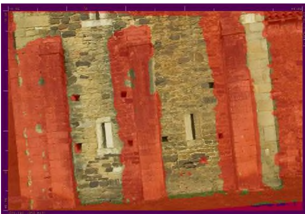
Figure 7. One image is mapped into another and matching is evident. Red areas have no disparity available from this pair
