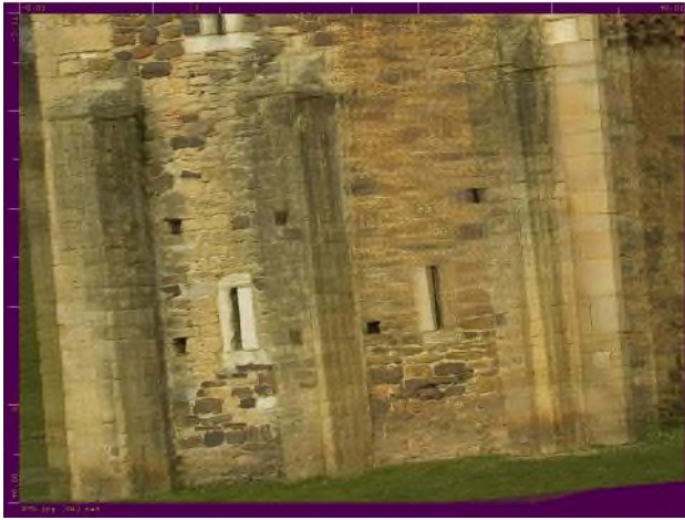
Figure 2. Two projections overlapped on the same single plane. Left window is closer to approximate plane, so looks sharper
