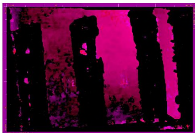
Figure 6. Disparity map detail of the lower part of a façade.
