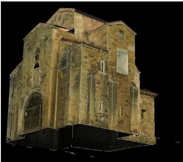
Figure 10. 3D model showing the planes used to approximate the surfaces
