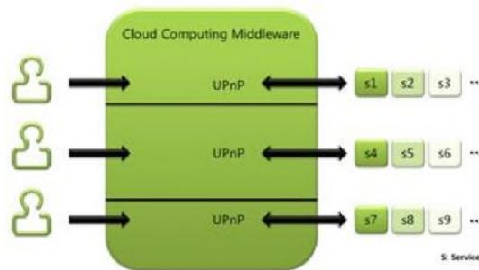
Fig. 2 Home network service architecture of cloud computing middleware
