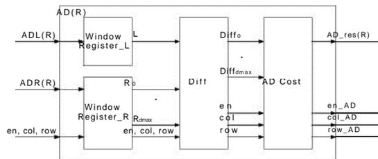
Fig. 2. Proposed AD core hardware architecture for red image.
