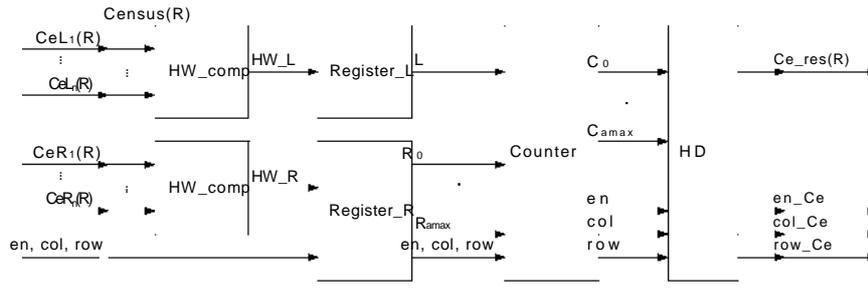
**Fig. 3.** Proposed Census core hardware architecture for red image.
