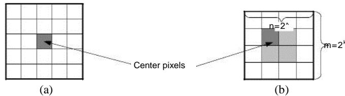
Fig. 1. Local matching windows: (a) conventional window, (b) proposed window.
