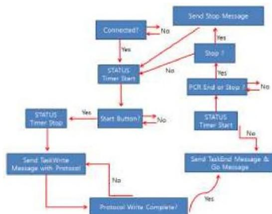
Fig. 2 Flow chart of the PCR control program
