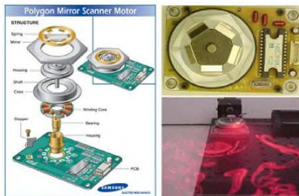
Fig. 2. Structure of general polygon mirror motor and sample of industrial use
